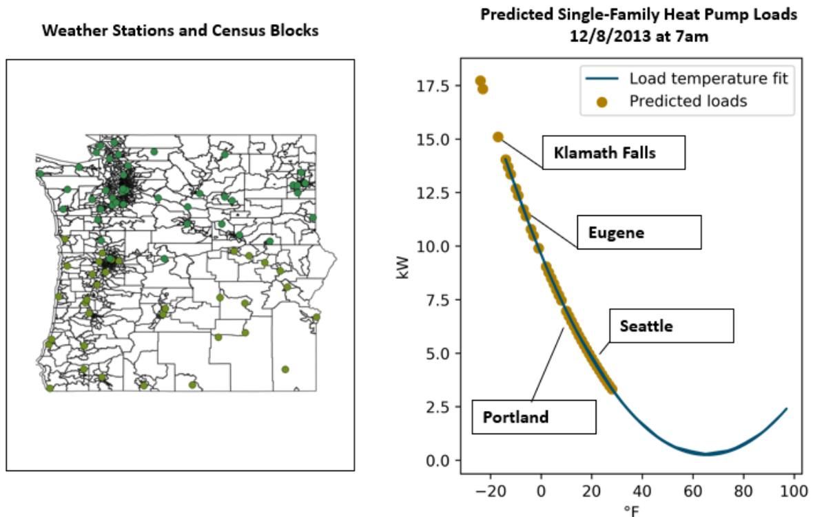
The average peak load for gas homes east and west of the Cascades simulated in Energy Plus during that hour was 6.8 kW. However, Washington was warmer than Oregon during that peak hour. As a result, the predicted loads using weather station data for Washington are 5.2 kW per home. In contrast, Oregon as
