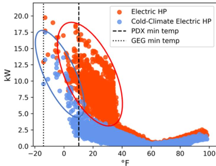
Big Ladder also simulated the performance of a cold-climate heat pump in a smaller home, comparing its hourly load with that of a conventional electric furnace. The heat pumps in these homes also require supplemental heat at temperature below 18° Fahrenheit but exhibit a large improvement in performance
