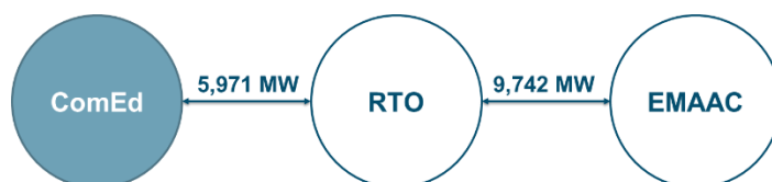
Figure 38: PJM Transmission Topology Modeled in RESOLVE
