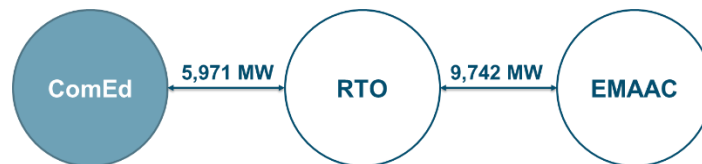
Figure 10: PJM Transmission Topology Modeled in RESOLVE
