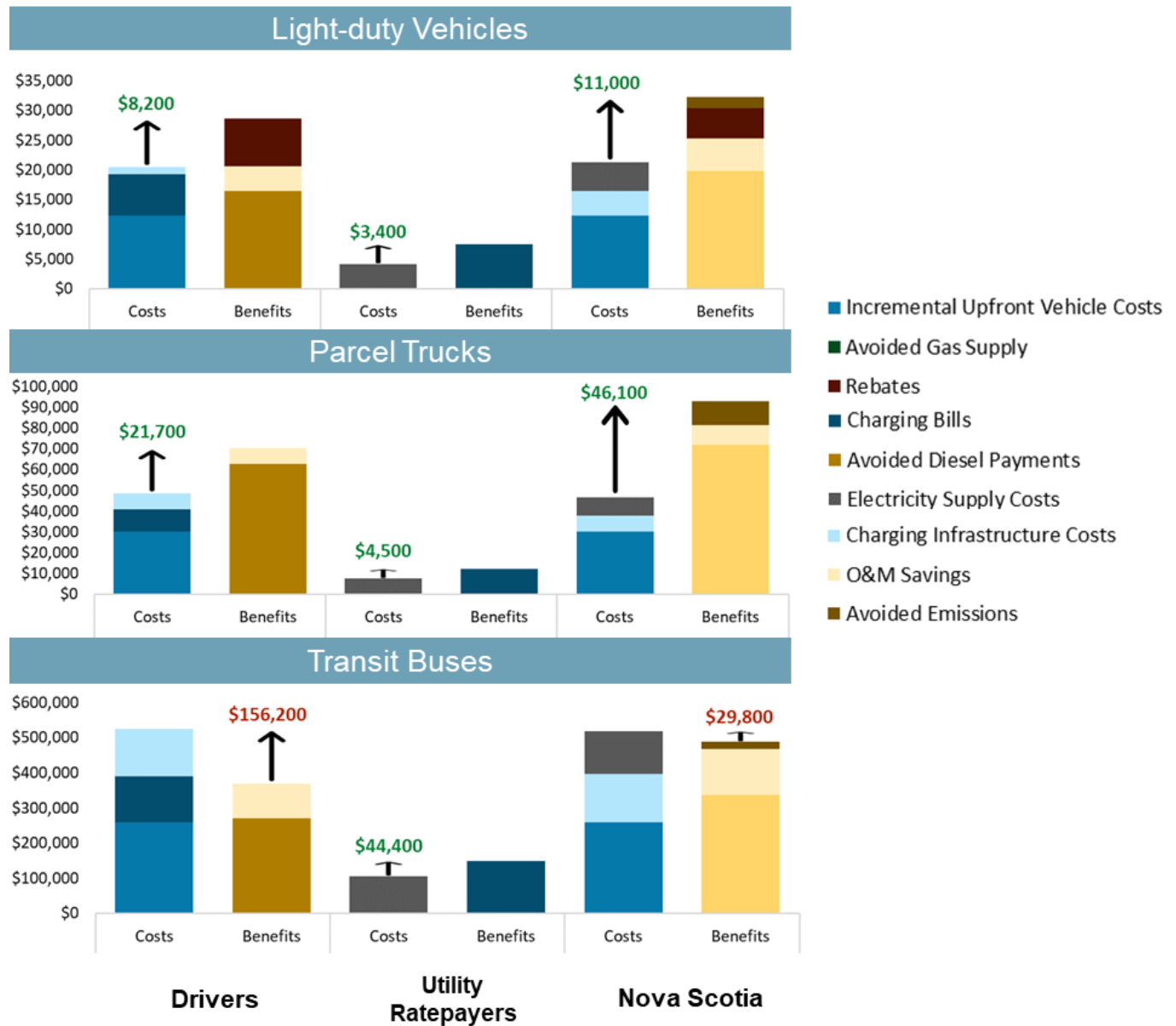
Figure 5-2. Net present value of costs and benefits of adopting light-duty vehicle in 2022, assuming managed charging with load management using vehicle-grid integration
